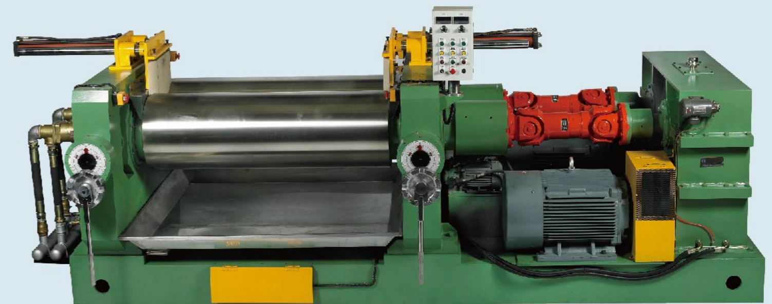
22寸雙馬達,雙輸出,速比自由調整,油壓檔板
